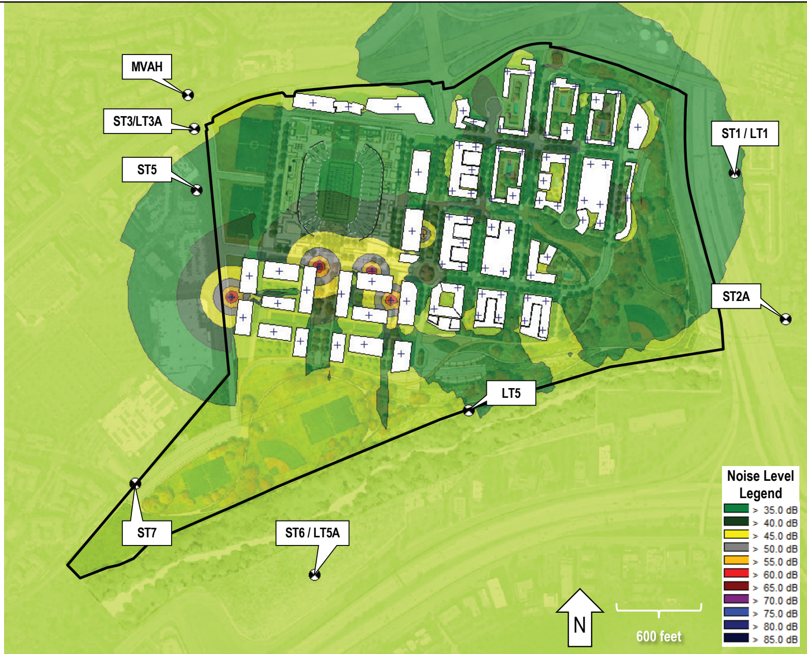
Figure 4.12-6 Predicted Project Stationary Operation Noise - Full Build-Out, without Stadium Event
